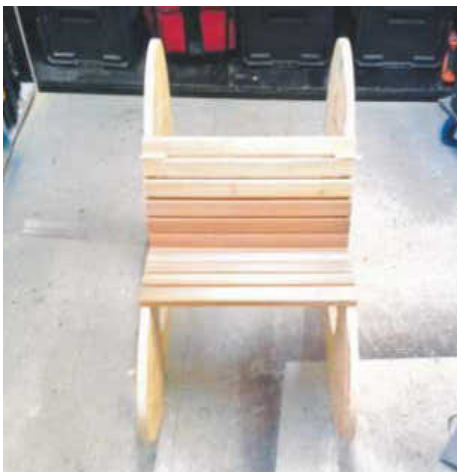
STEP 4. I also used window spacers to place between the cedar ribs so that the little gap between them is uniform all the way around
